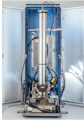
Bruker's latest member of the benchtop MALDI-TOF family, the smart-fleX, features both positive and negative ion mode allowing to access the full analyte space while spanning a wide mass range.
