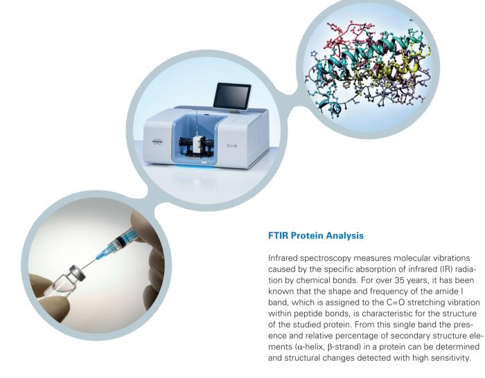
The CONFOCHECK is a dedicated Fourier transform infrared (FTIR) spectrometer system for protein analysis in aqueous solution.
