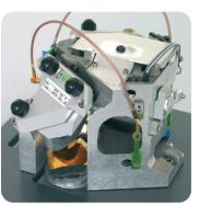
RockSolid™ interferometer used in the VERTEX 70v FT-IR spectrometer.
