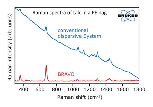
Raman spectra of talc in a PE bag measured with a conventional dispersive benchtop system and the BRAVO. BRAVO's SSE™ demonstrates efficient fluorescence mitigation and Duo LASER™ enables the detection of the weak Raman signals of talc with an exceptional signal to noise ratio.
