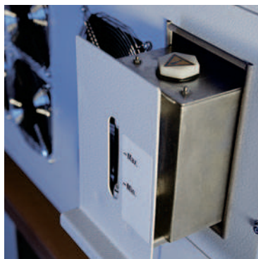
Internal water chiller
