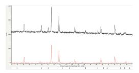
Unfiltered (black line) and filtered (red line) demonstrating the superb filtering of fluorescense radiation by the LYNXEYE XE-T.
