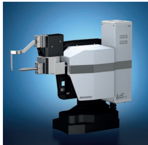
\mu S 3.0 X-ray source with Ag, Mo or Cu radiation
