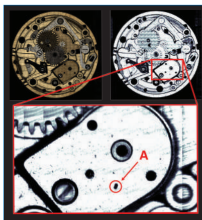
The visual image on the top left shows no indication of contamination or any presence of residue. The IR image at 1250 \text{ cm}^{-1} (top right) shows a small contamination. Size and extent of the contamination become clear in the close-up. The watch's entire movement ( 900 \text{ mm}^2 ) was analyzed in less than 5 minutes.
