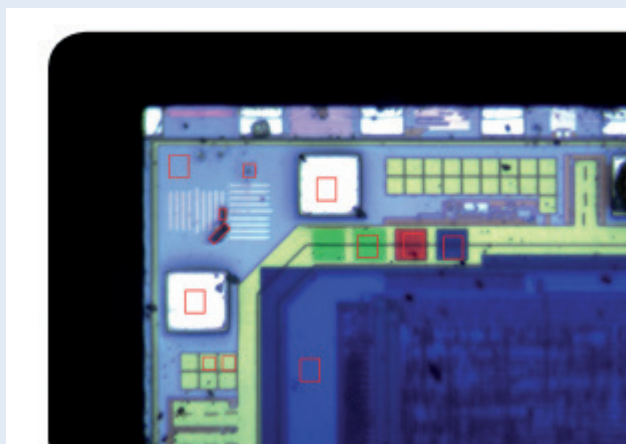
A CMOS chip of a digital camera was investigated by single point measurements to determine the cause of failure.
