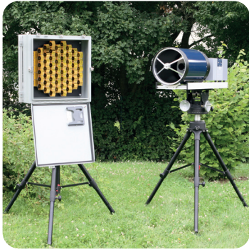
Open Path Monitoring System OPS
