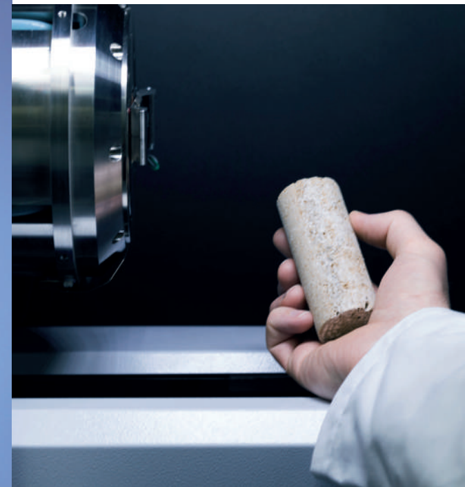
Large chamber for mounting big samples and optional stages
